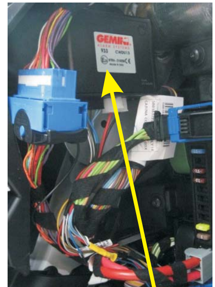
Fit the alarm unit over the top left corner of the fuse box.
