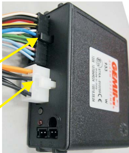
Plug the wiring harness connectors into the corresponding outlets on the alarm unit.
