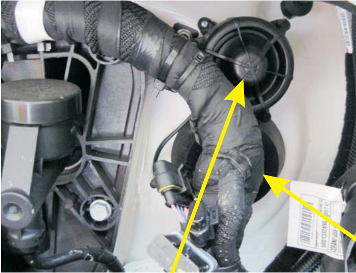
Fit the siren on the fireproof bulkhead, driver side, above the original grommet.
